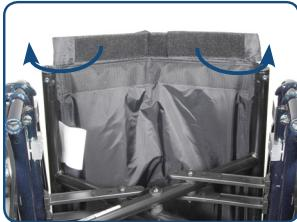
2. Pull outward on hook and loop straps to free them from underside of seat.
