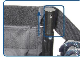
4. Pull outward on seat extension post until the second hole on the post lines up with the hole on the seat frame. Re-insert the screw into the seat upholstery and frame by turning clockwise to secure in place.
