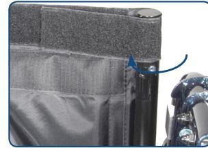
5. Fold hook and loop closure strap over extended seat post to secure seat upholstery to the frame.
